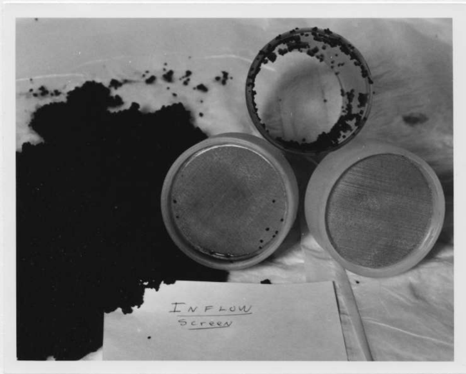
FIGURE 1. Photograph of carbon and cartridge components after perfusion and brief tap water rinse to remove blood. No clots, fibrin, or other evidence of blood intolerance was observed in the carbon, on the screen, or in the other circuit components. The inflow screen is on the left and is perfectly clean, as is the outflow screen on the right.
