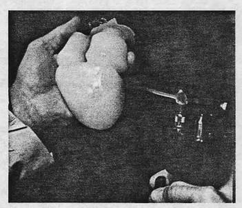
Figure 5. Flaming the Epolene.
