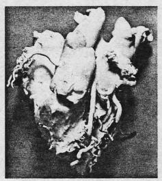
Figure 1. RTV mold of the natural heart.
