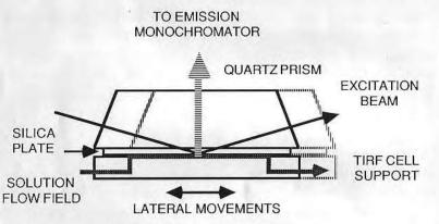
Figure 1. Schematics of TIRF cell with lateral scanning resolution.
