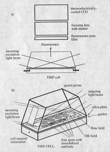
Fig. 1. Schematics of TIRF-CCD imaging of surface fluorescence: (a) optical arrangement of TIRF detection system, (b) the TIRF cell with four immobilized antibody spots and the outline of the excitation light path.
