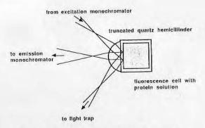
Fig. 1. Schematic illustration of TIRF cell geometry.
