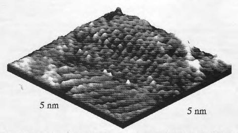
Fig. 3. The scanning tunneling microscopy image of LTI carbon surface from a heart valve disk. The STM probe was mechanically sharpened Pt/Ir wire, the bias tip voltage was 0·1 V and tunneling current was 1·0 nA. The surface was imaged in air.
