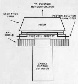
Fig. 3. Design of the TIRIF cell combined with  $\gamma$ -photon detector. The protein flow field is indicated.
