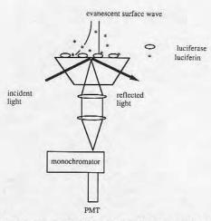
Fig. 1. A schematic picture of the TIRF cell and the optical geometry for the collection of surface fluorescence. The evanescent surface wave is not drawn to scale.
