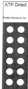
Figure 2 Current ATP platform sensor design based on a hydrophobic blue ink pattern deposited on a 1" x 3" microscope slide.
