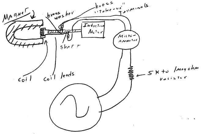
DiAgram of Apparatus and circuit used in the second Method described, this Method being much more accurate than the balance & light."
