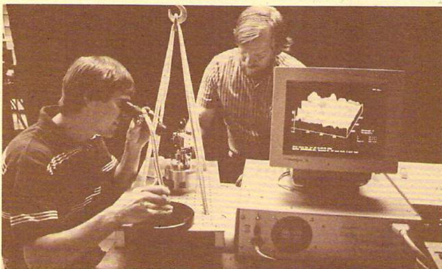
Bioengineering graduate student A. Scott Lea is mounting and adjusting a sample in the Atomic Force Microscope. Staff engineer Andras Pungor is providing helpful advice. A sample AFM image is on the screen.
