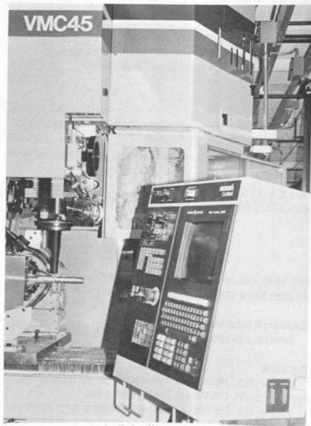
Five-axis computer controlled milling machine for computer-aided manufacturing (CAM) research.
